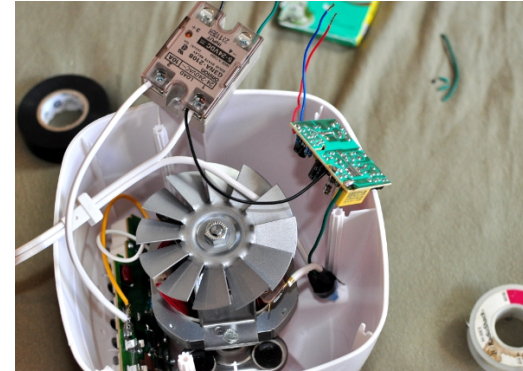
Figure 3: The innards of my hacked blender, with a relay and DC power regulation inserted.
