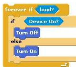
Fig. 2. This script allows any device to be turned on or off by clapping.
